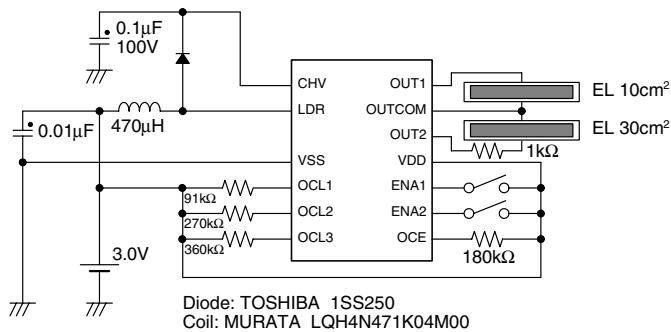
Note: Connect a 1kΩ resistor to protect IC when the EL is over 20cm<sup>2</sup> per channel.
