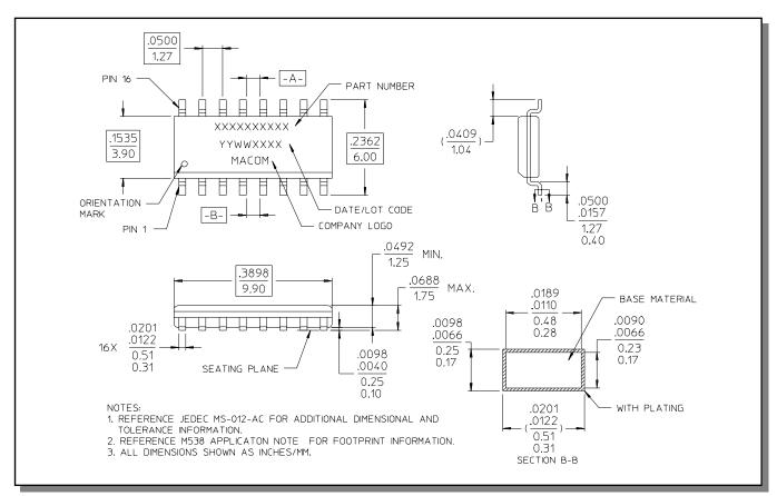
Reference Application Note M538 for lead-free solder reflow recommendations. Plating is 100% matte tin over copper.
