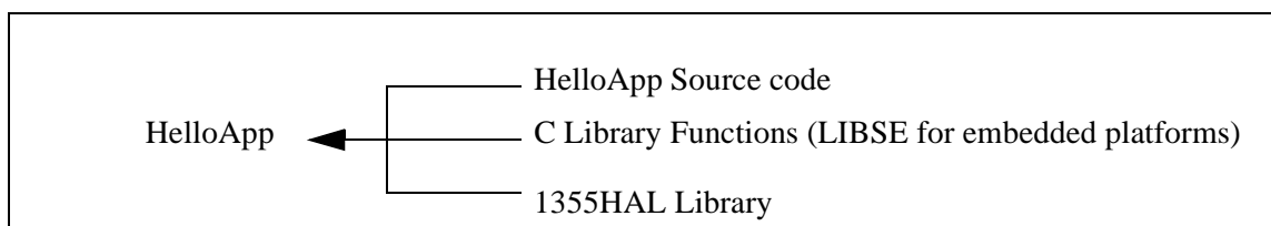
Figure 11-1: Components needed to build 1355 HAL application
