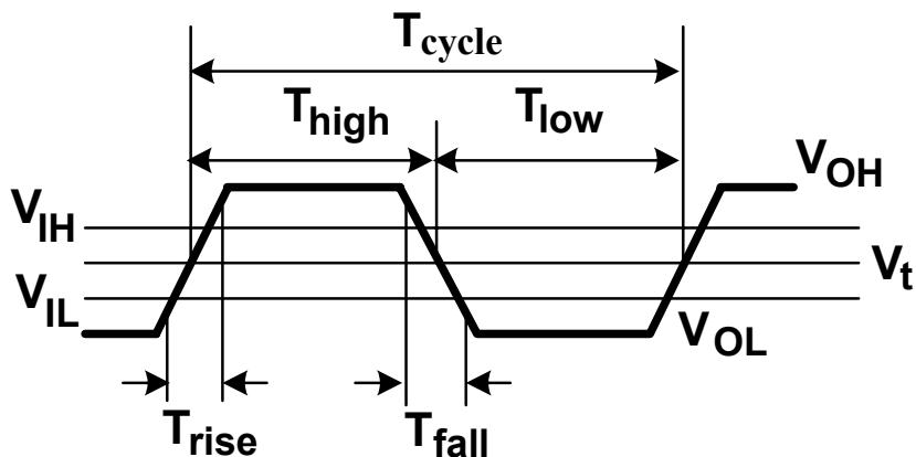
Figure 16. Output Timing
