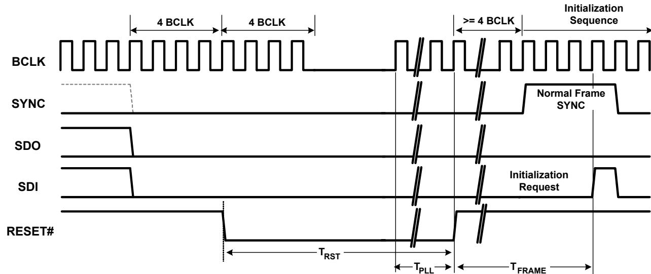
**Figure 14. Link Reset and Initialization Timing**
