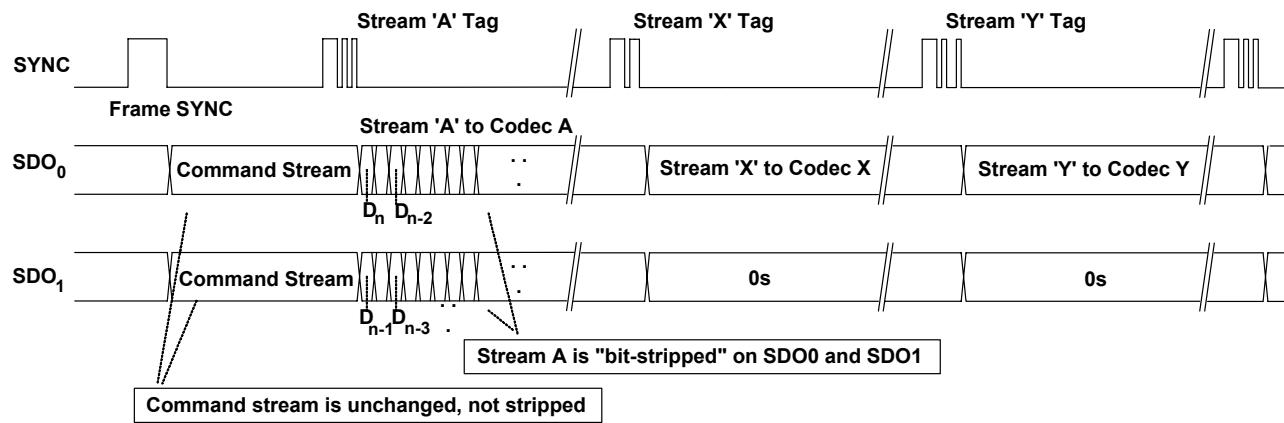
**Figure 8. Stripped Stream on Multiple SDO**
