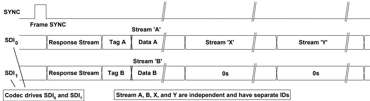
Figure 11. Codec Transmits Data Over Multiple SDI
