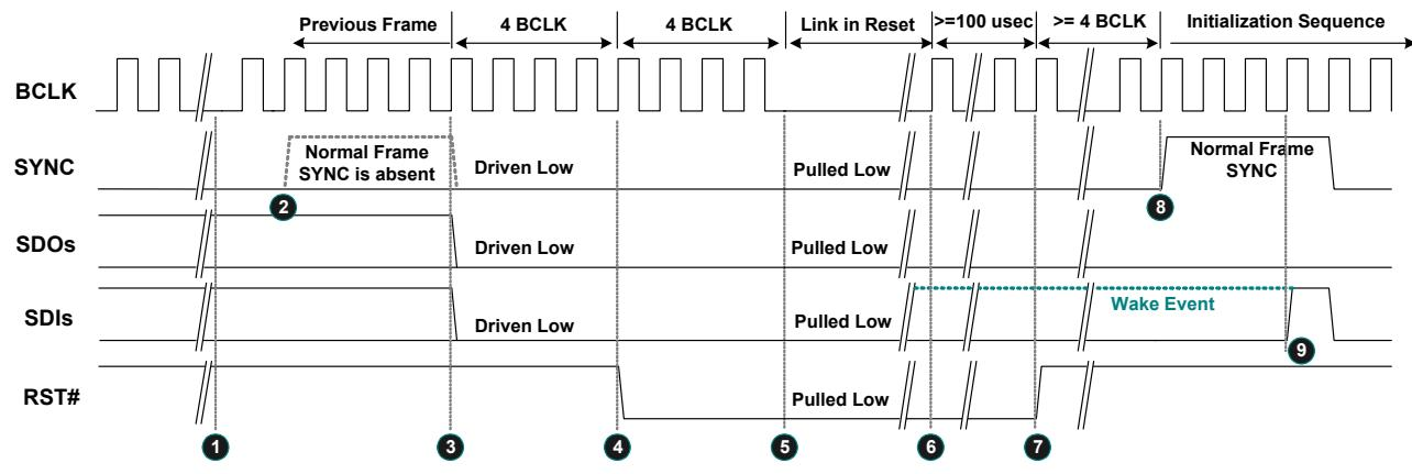
Figure 12. Link Reset Timing
