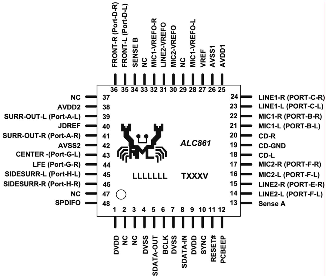
Figure 2. Pin Assignments
