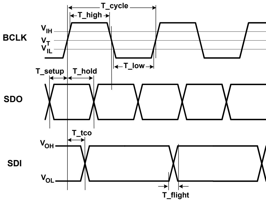
Figure 15. Link Signal Timing
