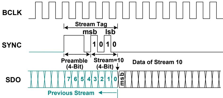
Figure 7. SDO Stream Tag is Indicated in SYNC
