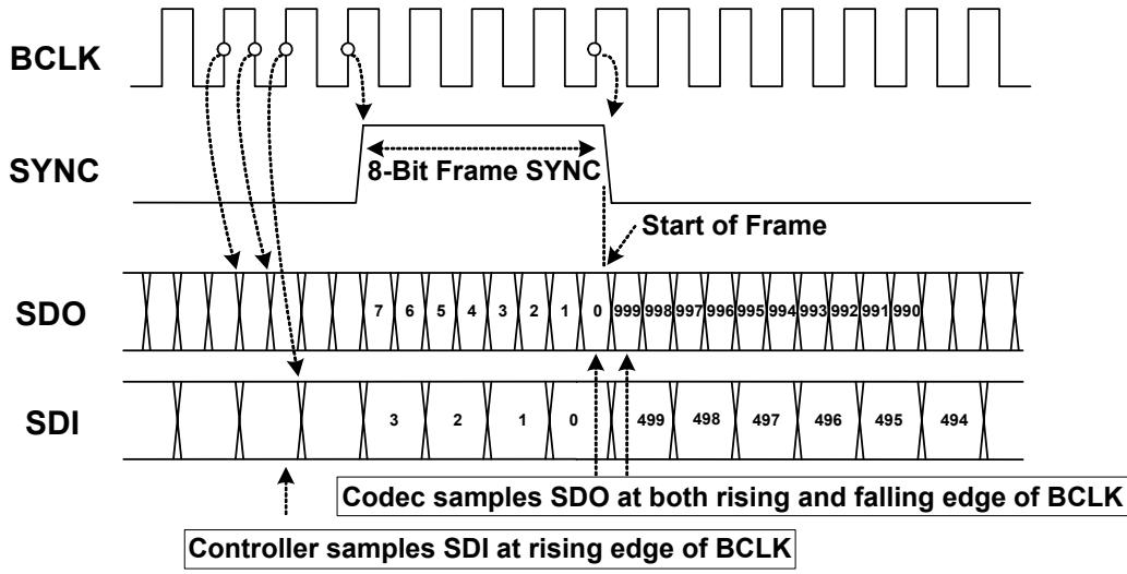
**Figure 4. Bit Timing**
