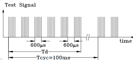
$T_{cyc} - T_d > 25 \text{ ms}$  is recommended for optimal function
