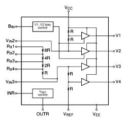
(This circuit must be used with  $V_{RX}1 \ge V_{RX}2 \ge V_{RX}3 \ge V_{RX}4$ .)
