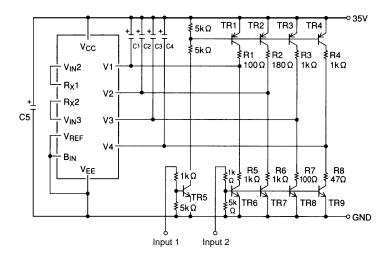
$$V_{CC}-V_{EE}=35~V,~R_X=8R,~C1~to~C4=10~\mu F,~C5=33~\mu F,~All~resistors~must~be~rated~1~W~or~higher.$$
