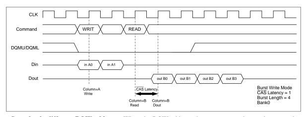
**Same bank, different ROW address:** When the ROW address changes, consecutive read commands cannot be executed; it is necessary to separate the two commands with a precharge command and a bank-active command.
