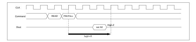
Write command to Precharge command interval (same bank): When the precharge command is executed for the same bank as the write command that preceded it, the minimum interval between the two commands is 1 cycle.
