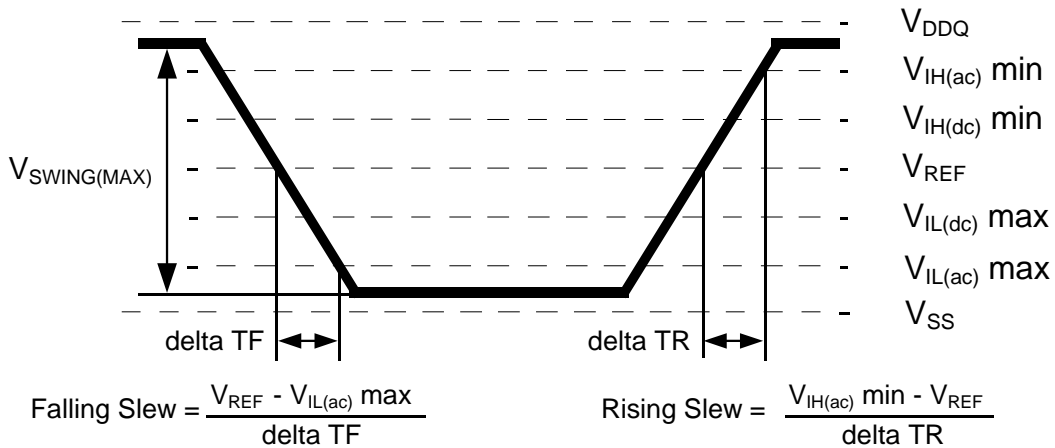
< Figure : AC Input Test Signal Waveform >
