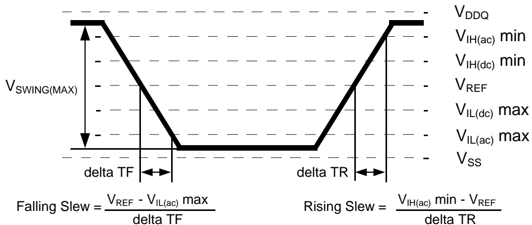
< Figure : AC Input Test Signal Waveform >
