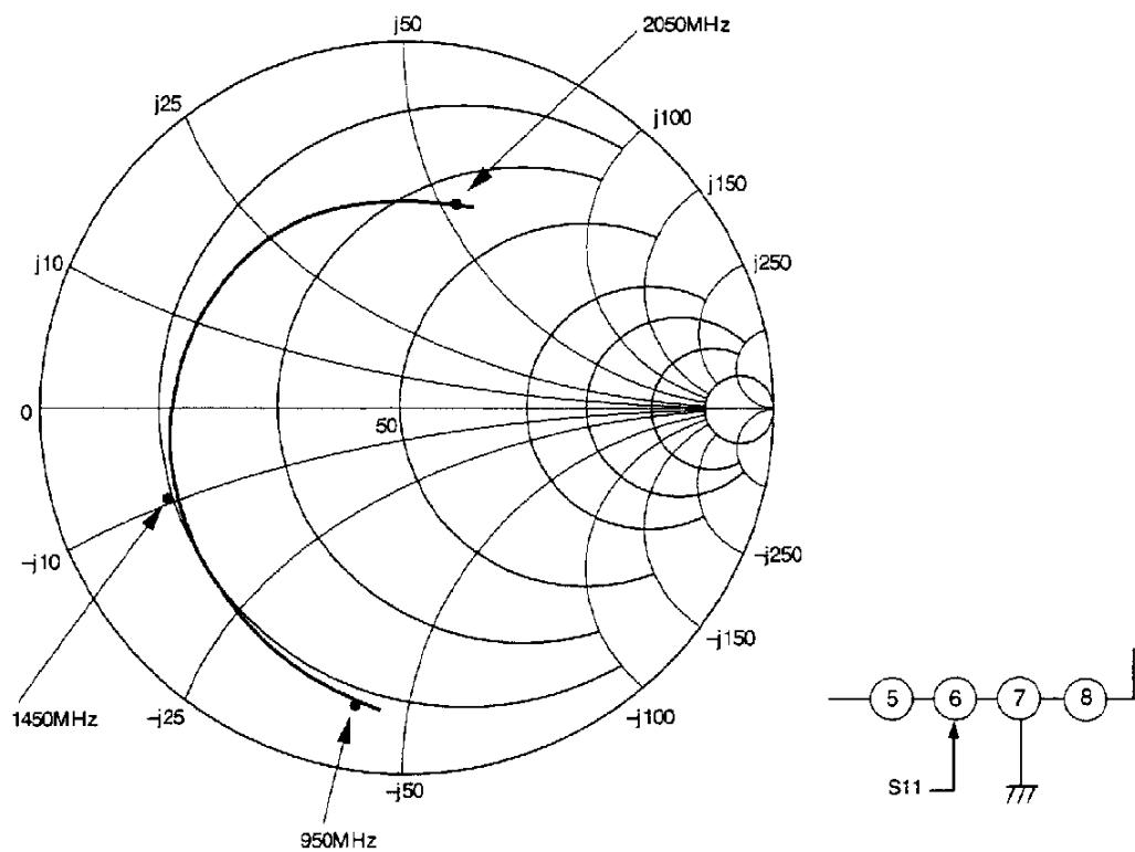
**Output Impedance (IF)**
