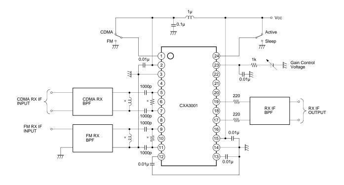
\* Must be adjusting values to result a best impedance matching between BPF filter and this IC.
