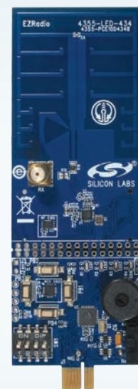
Si4355/Si4010 ONE-WAY SUB-GHZ KEY FOB TO LED RECEIVER STICK
