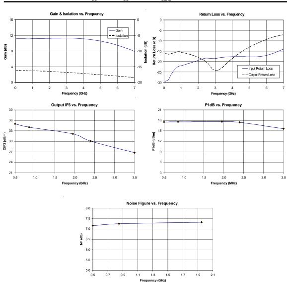
Typical RF Performance ( $V_{DS} = 5.3V$ ,  $I_{DS} = 65mA$ ,  $T_{LEAD} = 25^{\circ}$  C)
