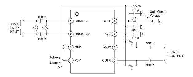
\* Must be adjusting values to result a best impedance matching between BPF filter and this IC.
