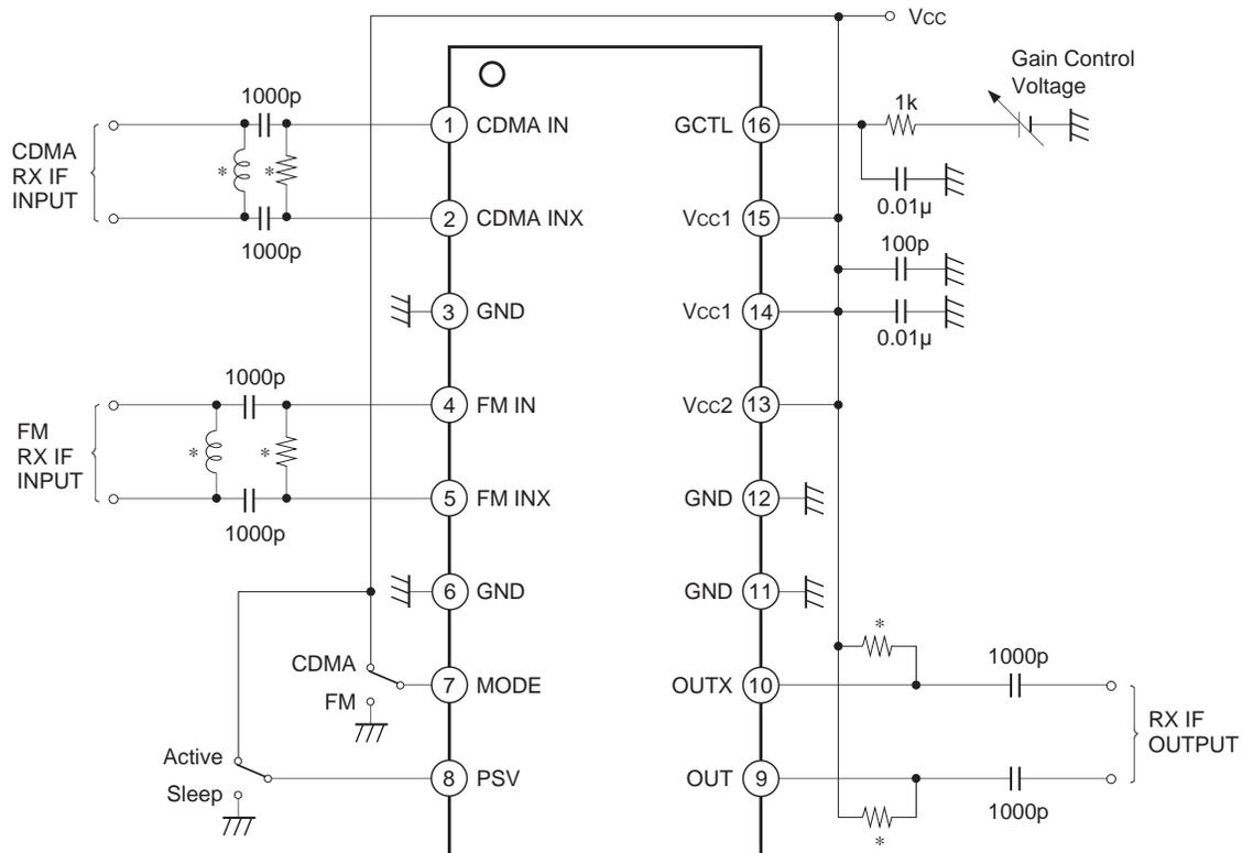
\* Must be adjusting values to result a best impedance matching between BPF filter and this IC.
