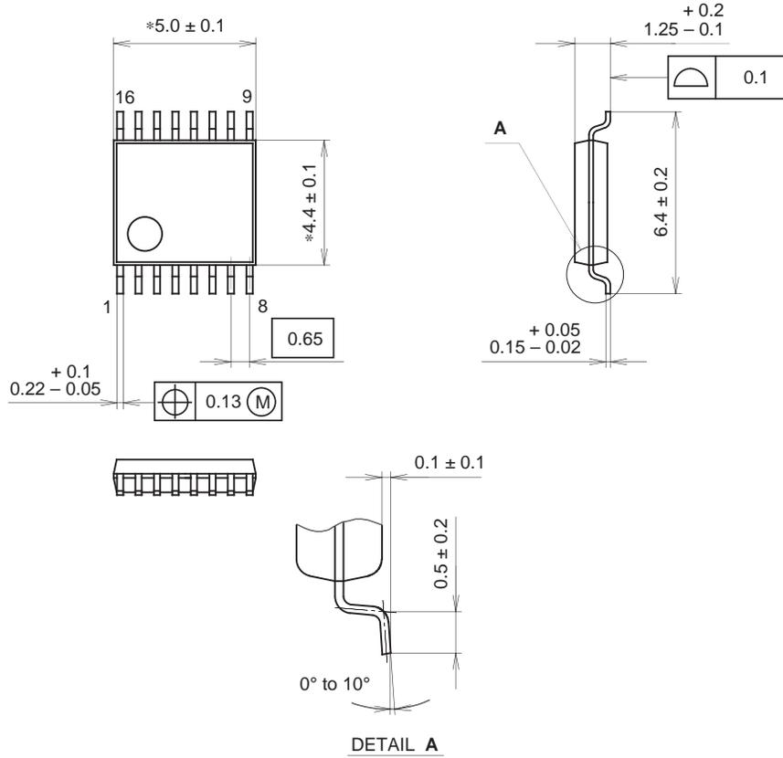
NOTE: Dimension "\*" does not include mold protrusion.
