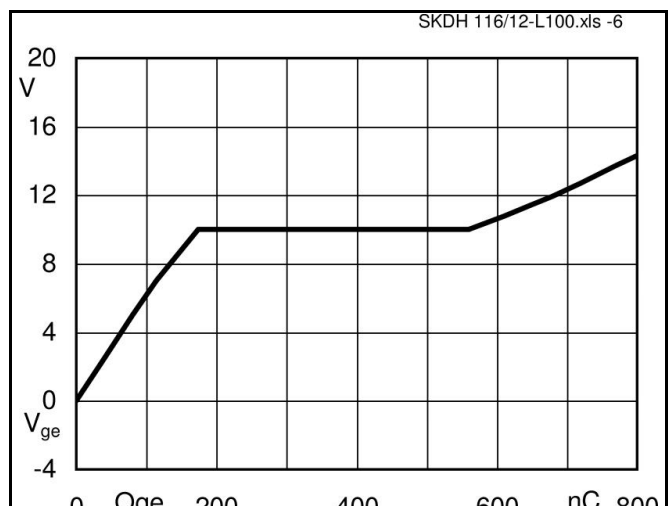
Fig. 6 Typ gate charge characteristic
