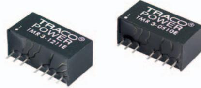
The TMR-3E series is a family of isolated 3 W dc-dc converter modules with regulated output, featuring wide 2:1 input voltage ranges. The product comes in a compact SIP-8 plastic package with small footprint occupying only 2.0 cm<sup>2</sup> (0.3 square in.) of board space.
