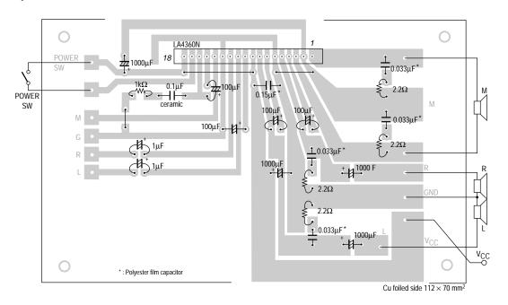
$\mbox{\ensuremath{\mbox{*}}}$  : Insert 0.15  $\mbox{\ensuremath{\mbox{\mu}F}}$  between power supply and ground at the root of the pins.
