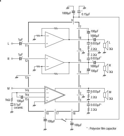
Note 1 : The motor should not be connected to the power switch pin since transient noise may appear on the amplifier outputs when the motor is started or stopped.
