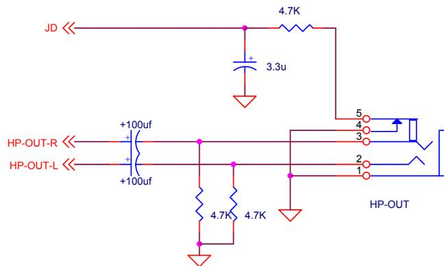
**Example of a Jack Detect Circuit**
