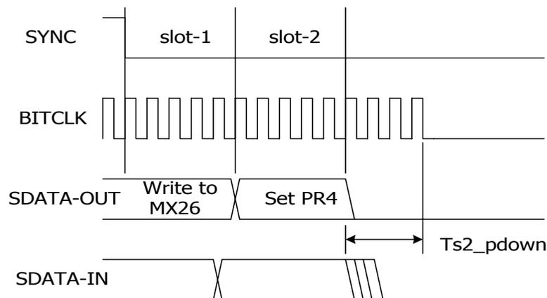
*AC-Link low power mode timing diagram*
