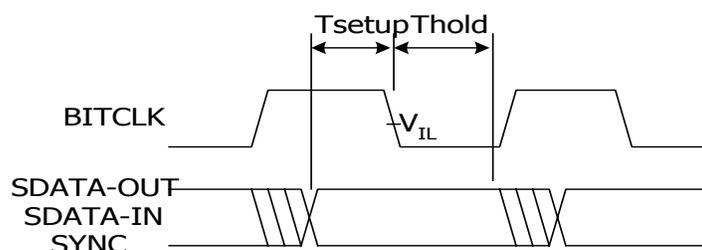
*Data Output and Input timing diagram*
