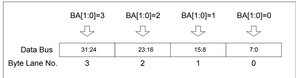
Figure 3-2. Little-Endian Mode Addressing
