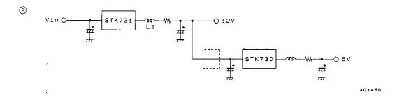
Note: It is possible for STK730 input ripple currents to cause L1 to vibrate audibly and adversely influence the 12 V system. If such problems occur, an inductor can be inserted at the point marked with dotted lines in the figure above to form an LC filter.
