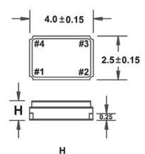
FX425A 0.8±0.1 (Resin Seal) FX425B 0.7±0.1 (Seam Seal)
