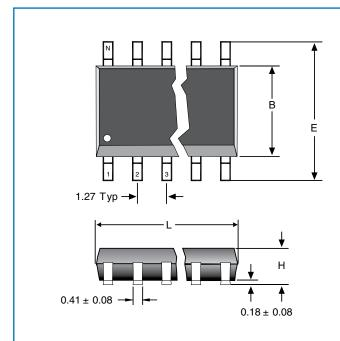
Note: All dimesions exclude mold flash and end flash which shall not exceed 0.15 per side.
