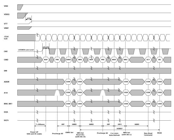
\* 200 cycle(tXSRD) of CK are required (for DLL locking) before Read Command
