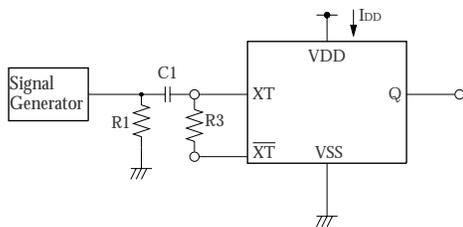
2.0V<sub>p-p</sub>, 70MHz sine wave input signal (3V operation)
