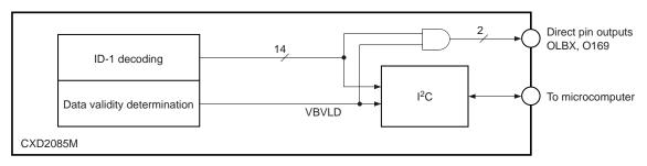
As shown in the figure above, the data validity determination which detects that the valid ID signal is exist or not, and the decoded result are obtained independently during ID-1 decoding. These two results are output to the direct output pins after taking their logical AND.
