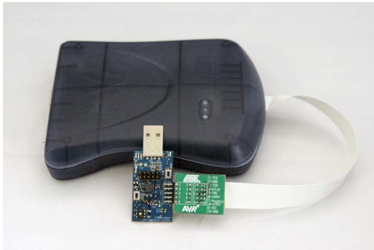
Figure 20. Connecting AVR JTAGICE mkII to the AT88Microbase
