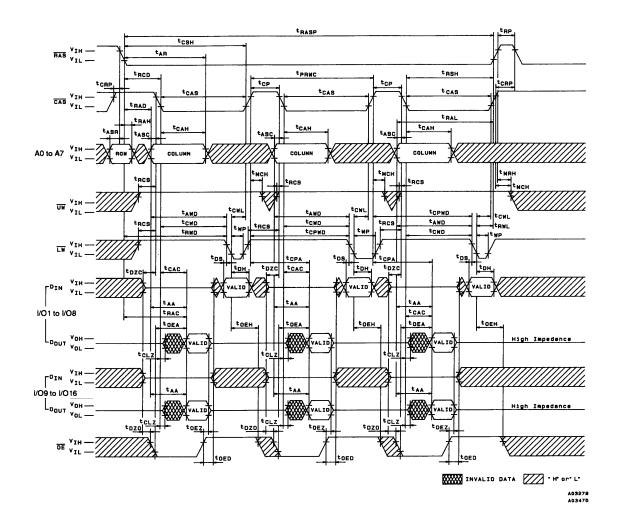
Fast Page Mode Read-Modify Lower Byte Write Cycle
