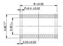
Recommended solder paste thickness: 120  $\mu m$
