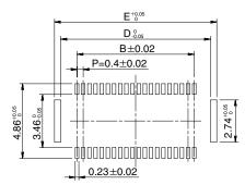
Recommended solder paste thickness: 120  $\mu m$
