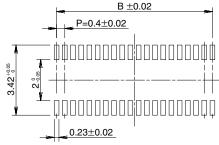
Recommended solder paste thickness: 120  $\mu \mathrm{m}$
