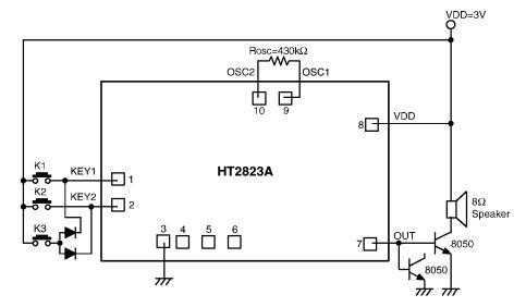
$\ensuremath{^{*}}$  The IC substrate should be connected to VDD in the PCB layout artwork.
