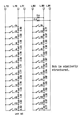
When data of -Ois transferred to main volume control 1dB STEP, S1,S2 are brought to open state and S3,S4 are turned ON simultaneously.
