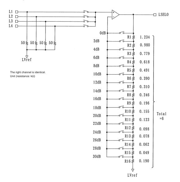
• Treble and bass band block internal equivalent circuit
