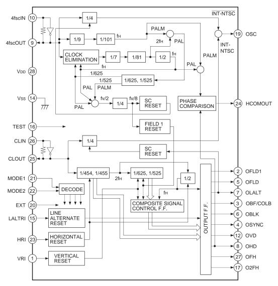
Note) Pin 19 output is (a) a signal based on Pin 26 in INT mode at NTSC. (b) each signal is based on Pin 10 in other modes.
