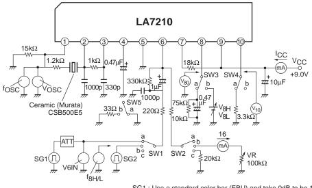
SG1 : Use a standard color bar (EBU) and take 0dB to be 1Vp-p. SG2 : Pulse generator (See the figure below.)
