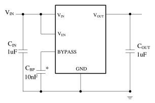
$C_{\text{OUT}}$ : Recommended ceramic capacitor
