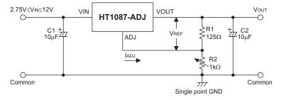
$$V_{OUT} = V_{REF} (1 + \frac{R2}{R1}) + I_{ADJ} R2$$
