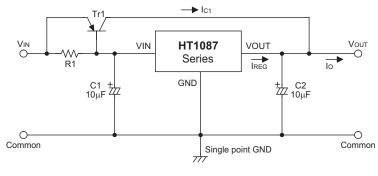
$$R_1 = \frac{V_{BE1}}{I_{REG} - \frac{I_{C1}}{(1+\beta)}}$$
