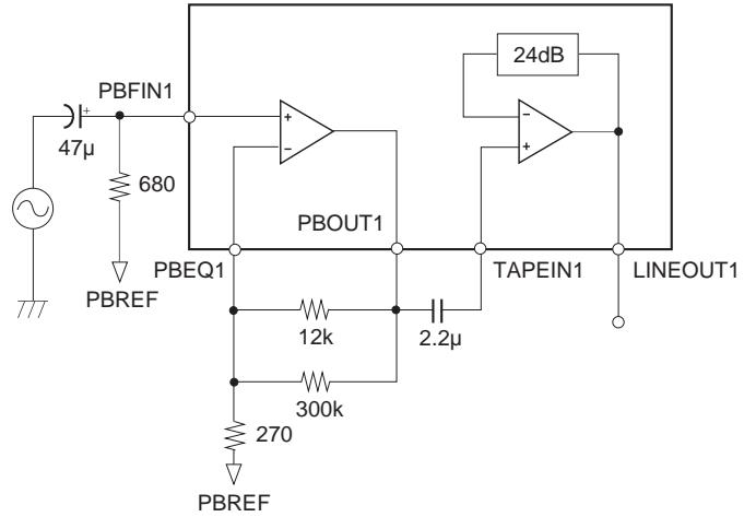
**Fig. 8. Measurement circuit of crosstalk between channels**
