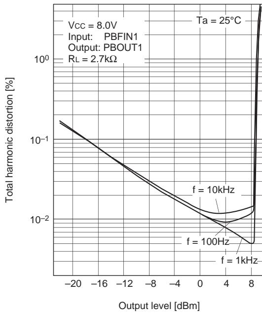
**B type total harmonic distortion (including NR OFF)**
