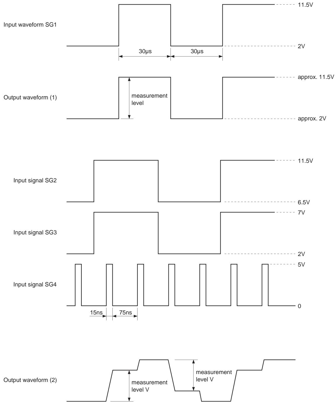
$$\text{Sample-and-hold slew rate} = \frac{V}{15 \times 10^{-3}}$$
