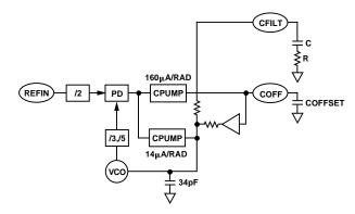
Figure 3b. Demodulator Block Diagram (Dmod Mode)
