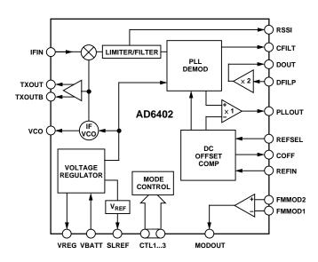
data output. On transmit, it accepts a Gaussian Frequency Shift Keying (GFSK) baseband signal, low-pass filters the signal if required using the on-chip op amp and modulates the IF VCO by varying the bias voltage on an off-chip varactor diode used in the tank circuit.
