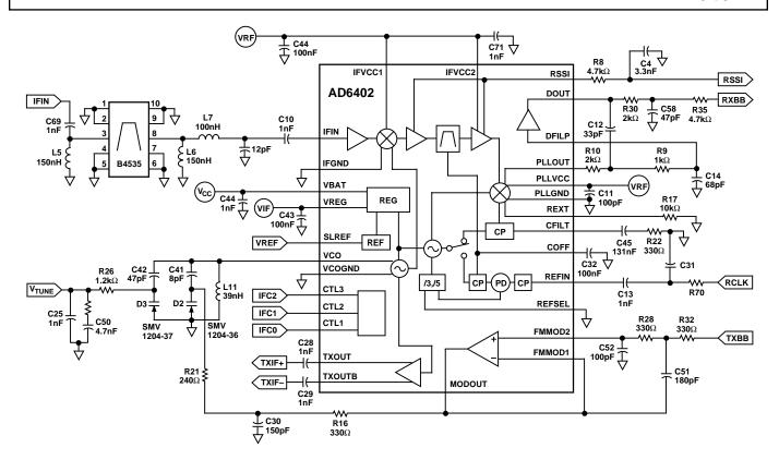
Figure 5. Application Circuit for DECT GFSK Transceiver
