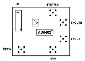
NOTE: SYNTH IN, TXOUTB, TXOUT, IFIN AND REFIN CONNECTED VIA SMA CONNECTORS
