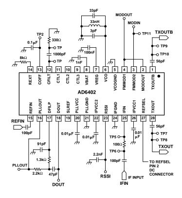
Figure 8. Evaluation Board Schematic
