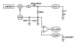
Figure 3a. Demodulator Block Diagram (Lock Mode)
