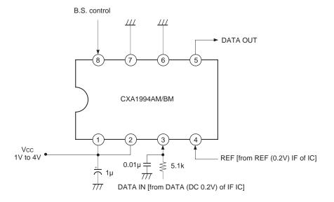
\* The comparator level can be set lower by inserting a resistor between Pin 1 (Vcc) and Pin 2.
