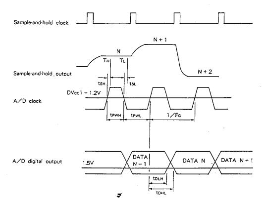
Th is the timing of latching result for the comparator of  $V_{N}$  and  $V_{REF}$  in the upper comparators. Tr is the timing of latching result for the comparator of  $V_{N}$  and  $V_{REF}$  in the lower comparators.
