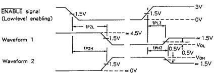
Output waveform of 3-state enable and disable time \*.
