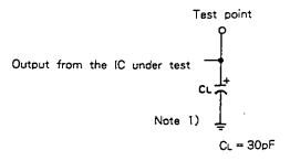
3-state Output Test Load Circuit
