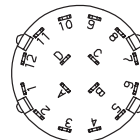
4P MODELS SP MODELS (omit terminals B, C & D) DP MODELS (omit terminals B & D)
