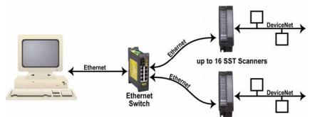
The SST Remote DeviceNet Scanner controls I/O devices connected to a DeviceNet network without the need of a local PC. DIN rail mountable, up to 16 SST Remote DeviceNet Scanners can be connected to one Ethernet switch which is then connected back to a PC residing on an Ethernet network. The PC allows users to remotely access diagnostic information on the SST Remote DeviceNet Scanner and the DeviceNet network.
