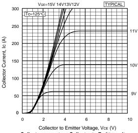
Collector current vs. Collector to Emitter voltage
