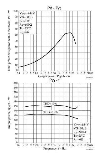
[Thermal Design Example for STK404-230-E (R<sub>L</sub>= $6\Omega$ )]
