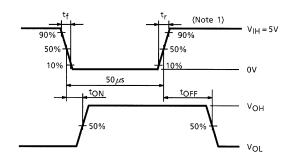
Note 1: Pulse width 50  $\mu$ s, duty cycle 10% Output impedance 50  $\Omega$ ,  $t_{\rm f} \le$  5 ns,  $t_{\rm f} \le$  10 ns
