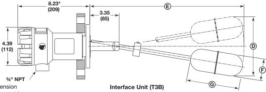
\* This dimension applies to cast iron housing. Subtract 0.31" for aluminum housing.
