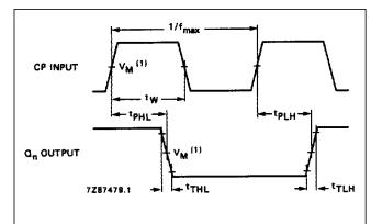
(1) HC :  $V_M$  = 50%;  $V_I$  = GND to  $V_{CC}$ . HCT:  $V_M$  = 1.3V;  $V_I$  = GND to 3 V.
