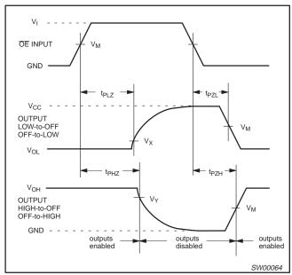
Waveform 2. 3-State enable and disable times
