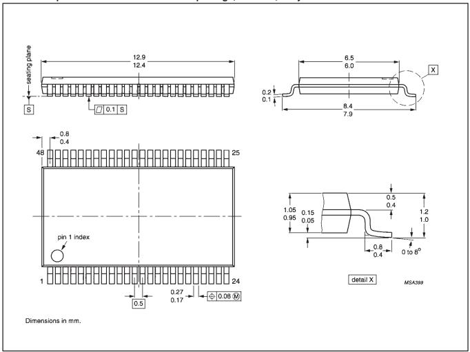
16-bit bus transceiver with direction pin;  $30\Omega$  series termination resistors; 5V Input/Outputs tolerant (3-State)
