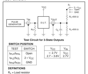
Waveform 3. Load circuitry for switching times
