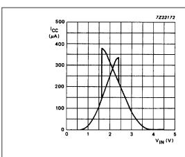
Typical HC transfer characteristics;  $V_{CC} = 4.5 \text{ V}.$
