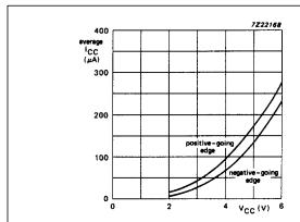
Fig.14 Average  $I_{CC}$  for HC Schmitt trigger devices; linear change of  $V_i$  between 0.1  $V_{CC}$  to 0.9  $V_{CC}$ .
