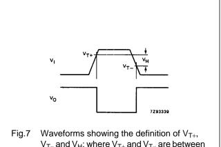
$V_{T-}$  and  $V_{H}$ ; where  $V_{T+}$  and  $V_{T-}$  are between limits of 20% and 70%.
