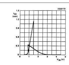
Fig.11 Typical HCT transfer characteristics;  $V_{CC} = 4.5 \text{ V}.$
