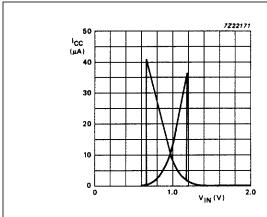
Fig.8 Typical HC transfer characteristics;  $V_{CC} = 2 V$ .
