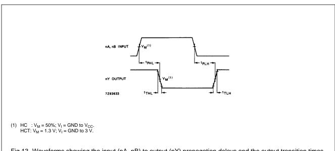
Fig.13 Waveforms showing the input (nA, nB) to output (nY) propagation delays and the output transition times.
