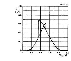
Fig.10 Typical HC transfer characteristics;  $V_{CC} = 6 V$ .
